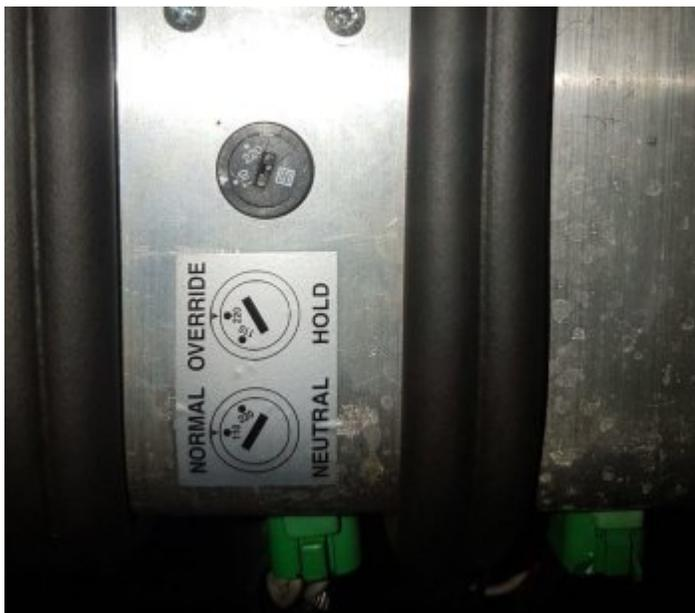
**Note** The motorhome will not go into gear if the room is not fully retracted but if it is a false signal, you can override by going to the bay with the pump and turn the servo to "220". Use a screwdriver, top right hand corner of bay.
