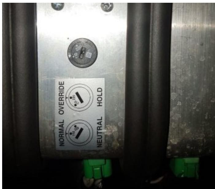
**Note** The motorhome will not go into gear if the room is not fully retracted but if it is a false signal, you can override by going to the bay with the pump and turn the servo to "220". Use a screwdriver, top right hand corner of bay.
