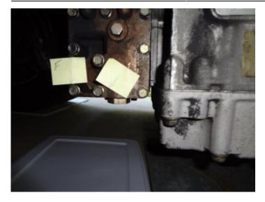
I noticed an occasional small drop of "oil" on the floor beneath the back of the transmission. It concerned me so I had mechanics and technicians look at it. I had checked fluid level, no detected loss.
