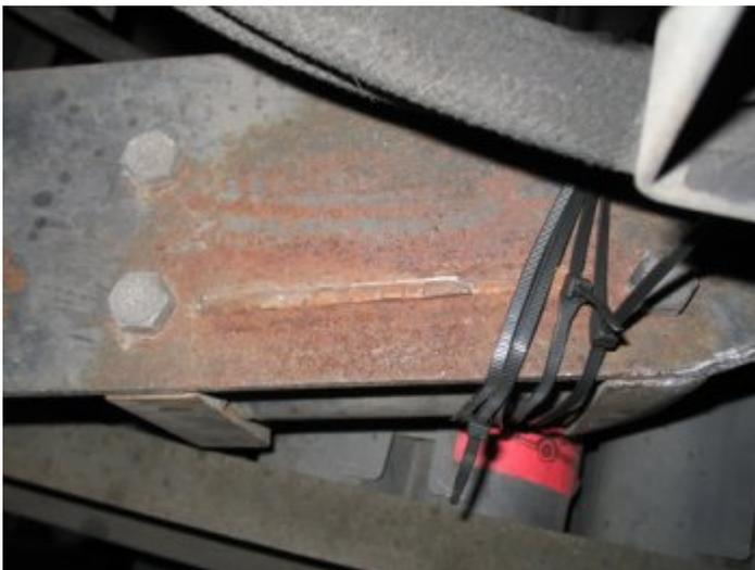
Shows where the metal fractured
