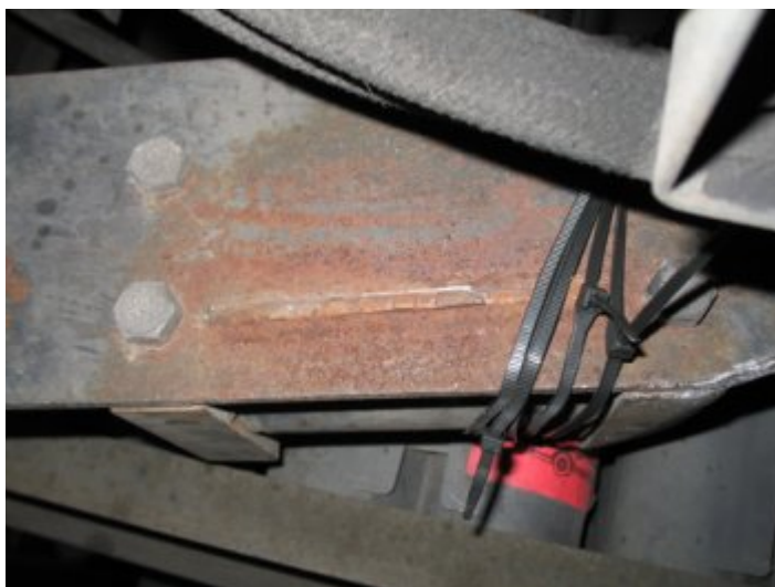
Shows where the metal fractured
