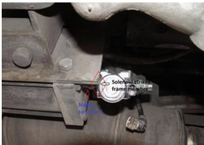
The solenoid on the new assembly is a little wider than on the old one Part #29522717. As a result, reusing the old nipple did not work. I had to get something longer. Found a 3/8" x 2" nipple at the local auto parts store, which worked fine.
