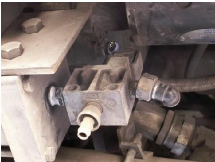
Removal is pretty easy; disconnect air supply line and the electrical connector.
