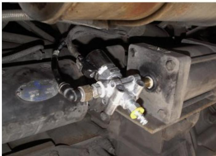
I used a TFE thread sealer. Tested for leaks with soapy solution; none found.
