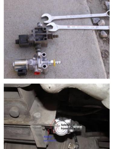
The solenoid on the new assembly is a little wider than on the old one Part #29522717. As a result, reusing the old nipple did not work. I had to get something longer. Found a  $3/8" \times 2"$  nipple at the local auto parts store, which worked fine.
