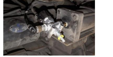
I used a TFE thread sealer. Tested for leaks with soapy solution; none found. Now we just have to confirm normal operation of the retarder on our next trip in a couple weeks.
